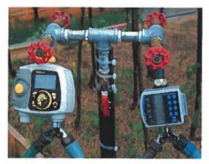
Figure 6. Irrigation timers.
